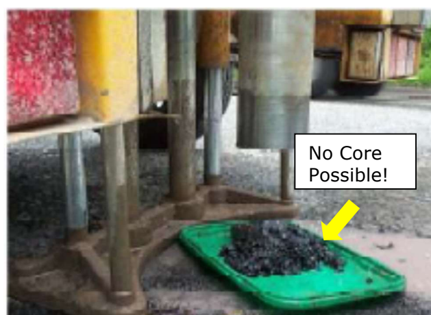
Alternative HAPAS approved PCSM – Coring attempt made 24 months following compaction. Coring carried out by Surry CC materials Laboratory
