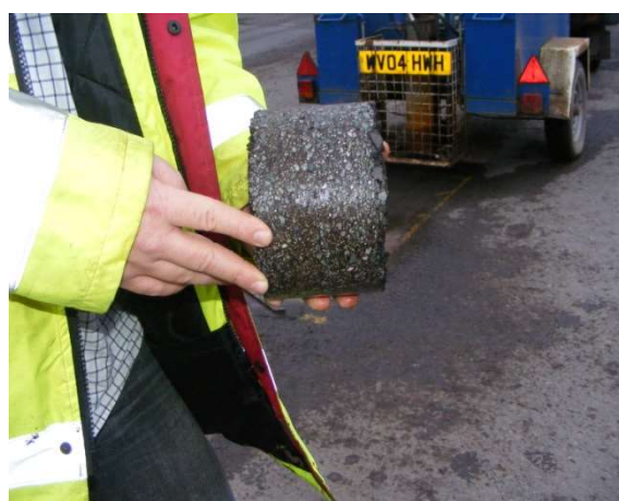
Viafix core – taken just 24 hours following compaction
